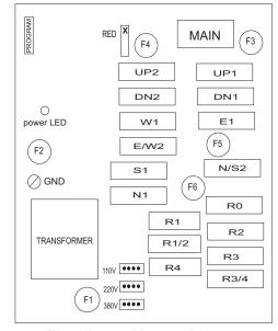
Fig. 1 Internal Layout Diagram
